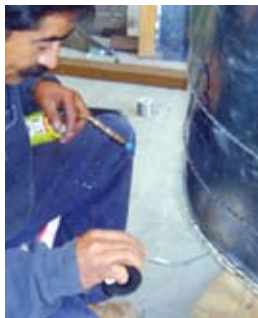
Figura 51. Soldar la base.
