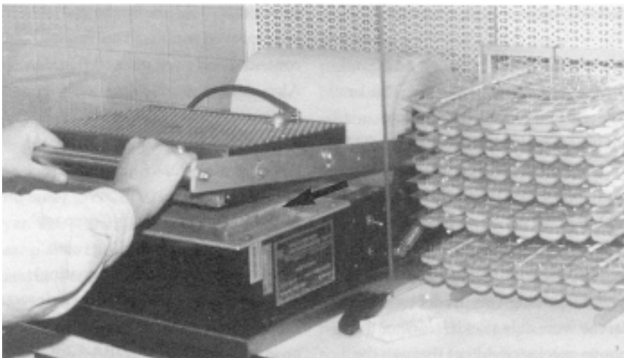
Figure 2. Semiautomatic lidder to seal Mylar® film to the top of the plastic tray.
