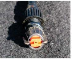
Flat fan nozzles are the recommended nozzles to apply glyphosate with a knapsack sprayer
