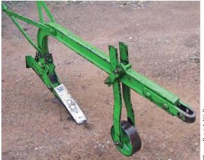
The Magoye ripper mounted on a plough frame can be used to open small furrows for hand seeding.
