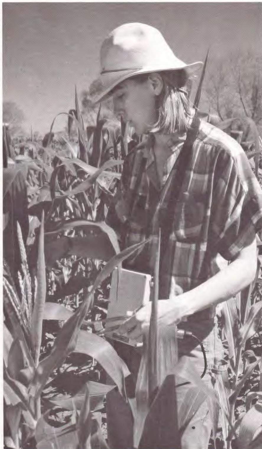
Associate scientist Renée Lafitte uses a portable photometer to measure chlorophyll content (an indicator of nitrogen status) as part of a program for improving nitrogen-use efficiency in maize grown under low supply of this nutrient.
