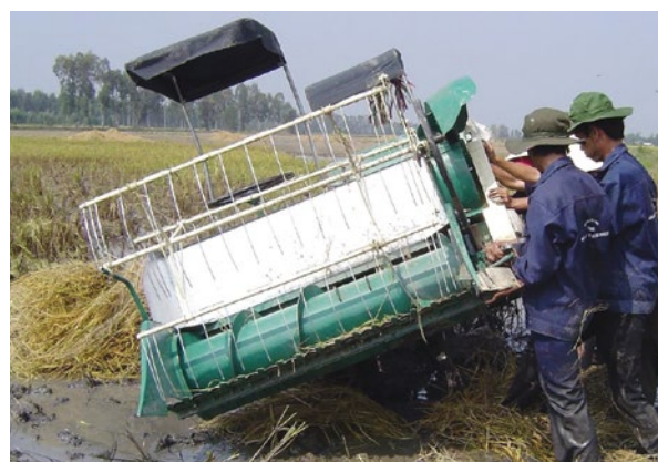
Figure 31. This type of combine is easily lifted for changing its wheels.
