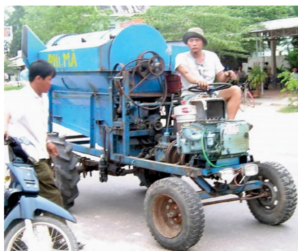
Figure 28. The self-propelled type axial-flow thresher.
