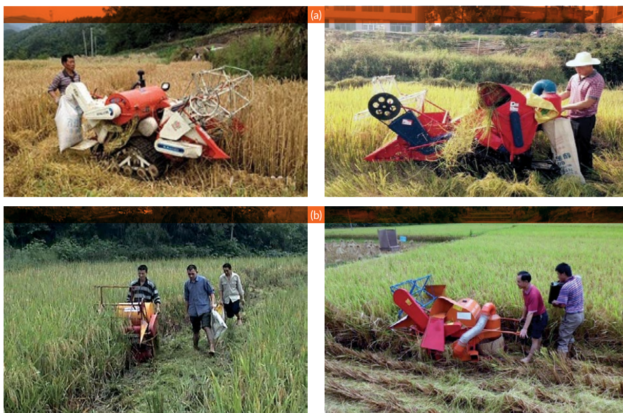
Figure 54. Crop residue management with mini combines (a) in wheat fields and (b) in rice fields. (Source: Baidu).
