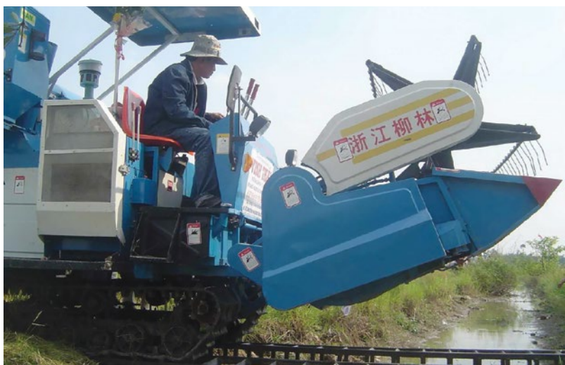
Figure 33. A 2 tonne combine crossing a canal on metal frames.
