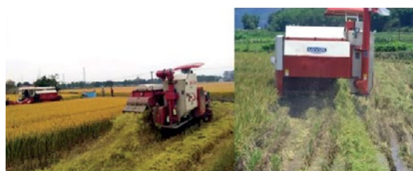
Figure 52. Stacking method of stubble under small combine harvesting with evenly distributed straw (left) and windrowed straw for recycling (right).
