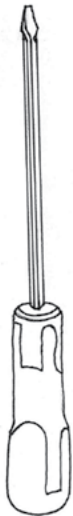
Screwdriver (flat head): used to screw in or out screws with a – shape at the head of the screw.
