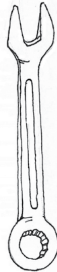
Dull wrench: Used to turn bolt heads to the left or right. This one has two ends, the circular end has the best grip.
