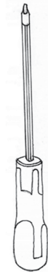
Screwdriver (star/Phillips head): Used to screw in or out screws with a + shape at the head of the screw.
