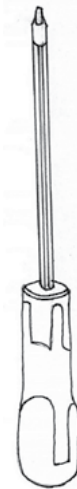
Screwdriver (star/Phillips head): Used to screw in or out screws with a + shape at the head of the screw.
