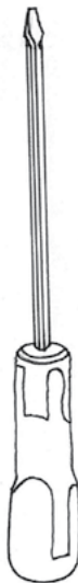
Screwdriver (flat head): used to screw in or out screws with a – shape at the head of the screw.
