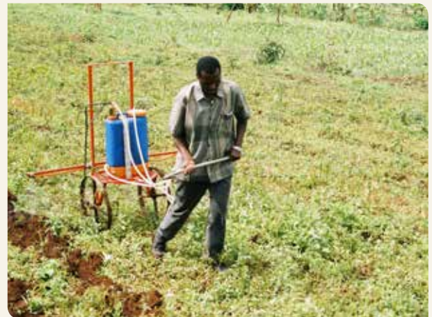
Plate 1.7 Backpack sprayer adapted to wheeled frame and pulled behind the operator © B. Sims
