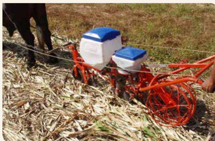
Plate 1.3 Animal-drawn no-till planter with double offset disc openers © B. Sims
