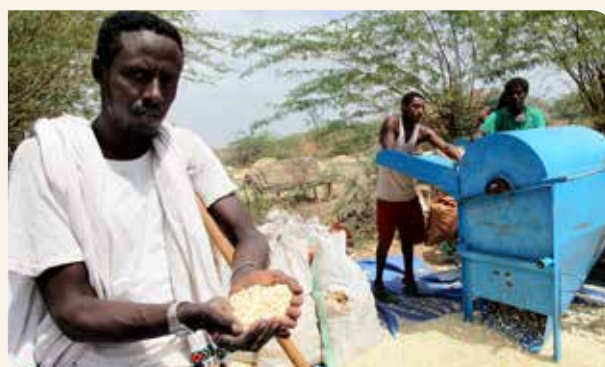
Plate 1.11 Engine-powered maize sheller ©FAO / T. Legesse
