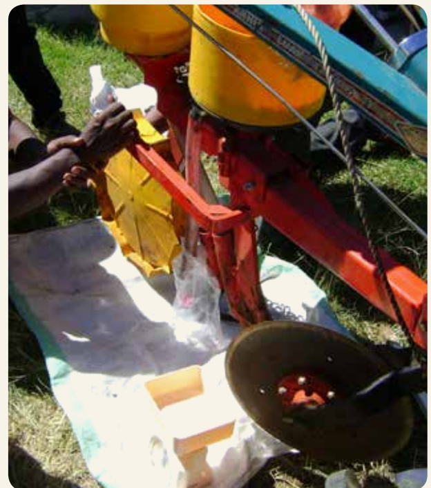
Plate 4.10 Calibration of seed delivery for a 2WT-drawn no-till planter © B. Sims
