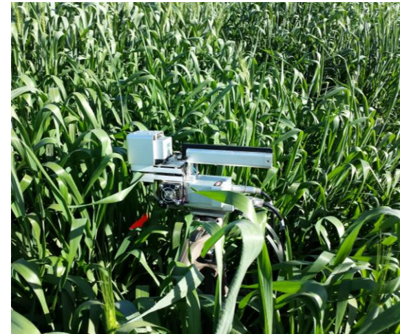
Gas Exchange: A/Ci curve (30-45 min)
