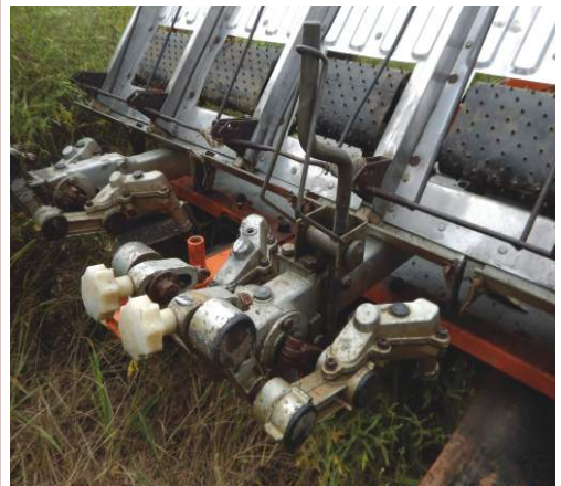
Planting Depth Control : (a) Sliding lever (b) Rotatory lever
