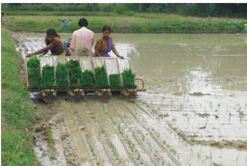
Mechanical transplanting of rice : a suitable and profitable alternative to manual transplanting
