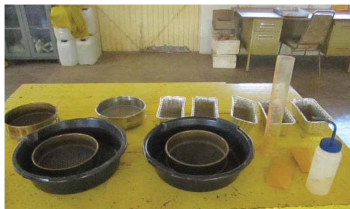
Figure 5: Setup for the alternative sieving method.
