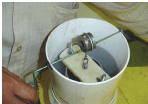
Figure 3. Immersion of the stack of sieves in distilled water.
