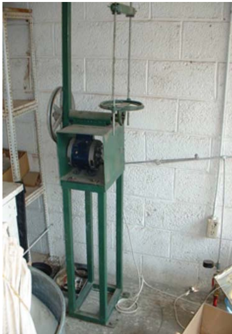
Figure 1. Machine used to shake dry soil samples.
