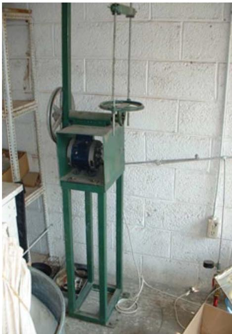
Figure 1. Machine used to shake dry soil samples.
