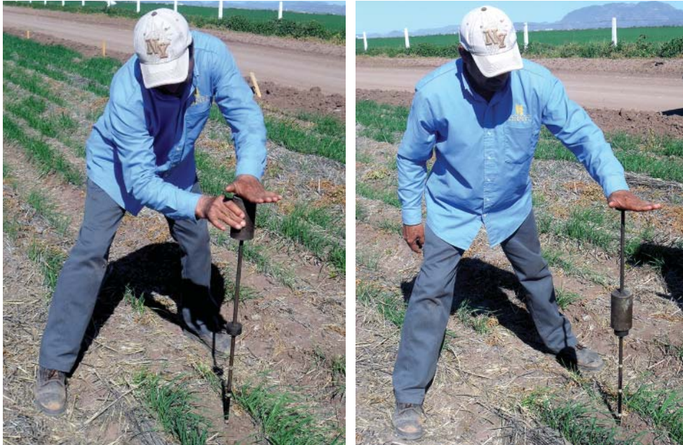
Figure 1. Use of the penetrometer: Left: the weight is raised all the way to the top of the penetrometer; Right: the weight is dropped and one impact is counted.
