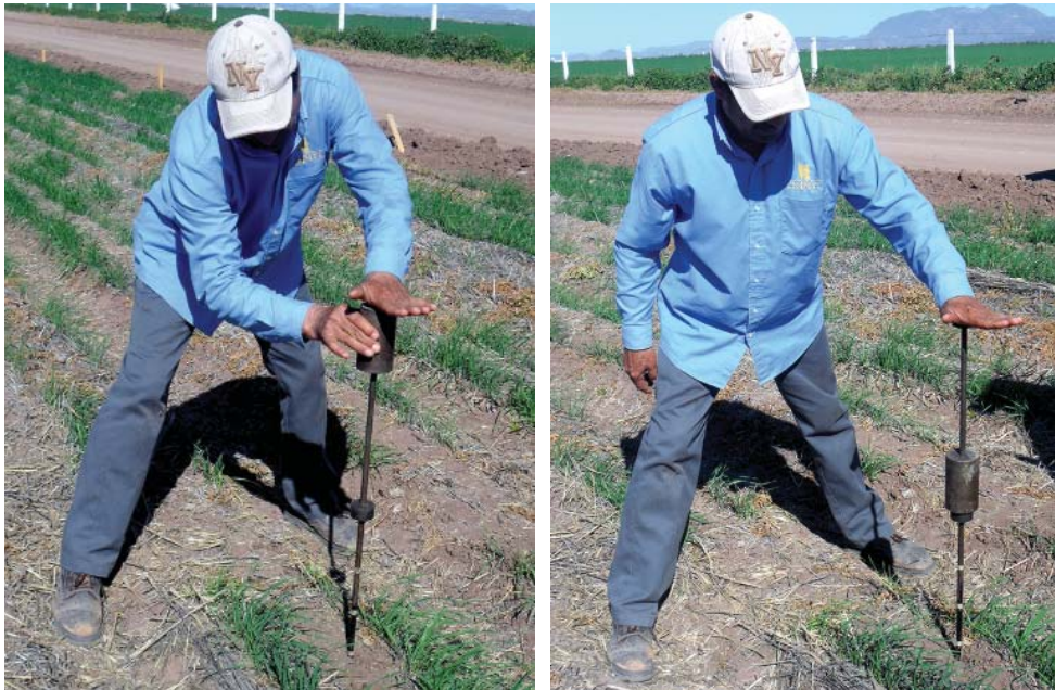
Figure 1. Use of the penetrometer: Left: the weight is raised all the way to the top of the penetrometer; Right: the weight is dropped and one impact is counted.
