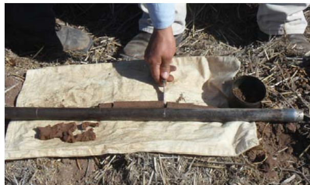
Figure 2. To improve efficiency more than one sampling depth can be sampled at once. This involves spreading the sample onto a piece of cloth or plastic and using the probe as a ruler to divide the sample into the correct fractions.
