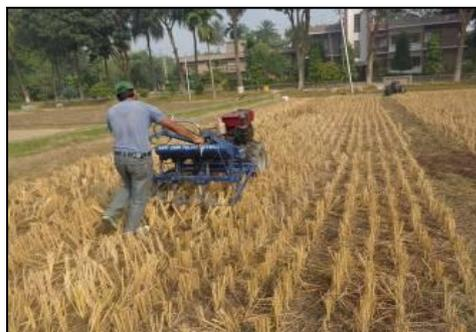
**Fig. 1. 2WT operated no till seeder**
