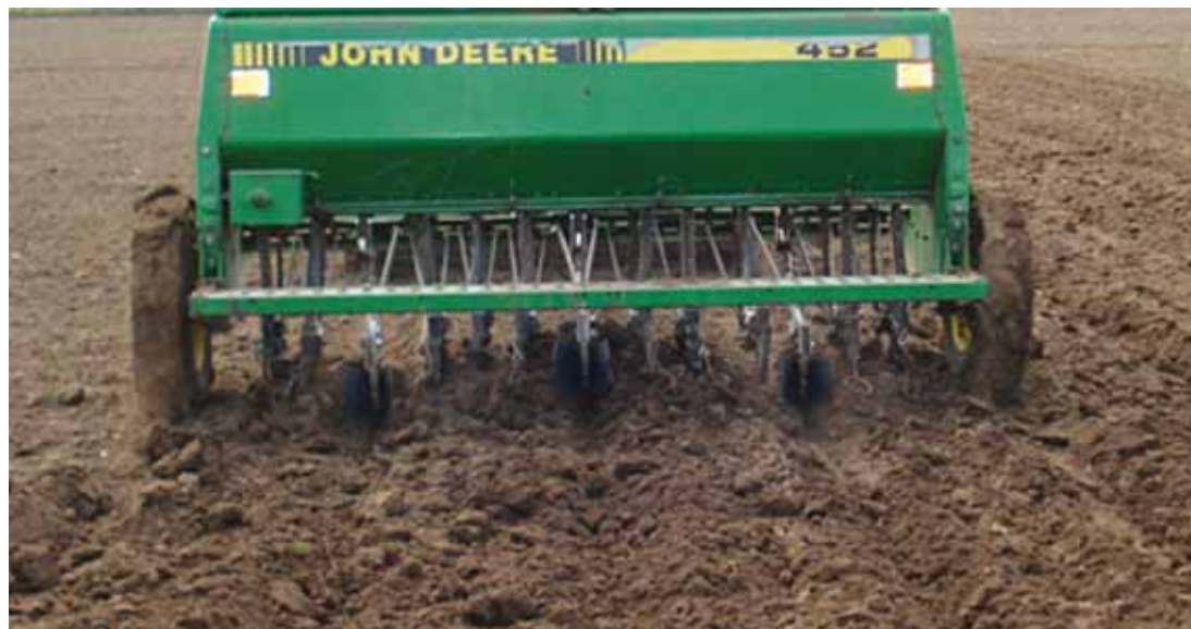
Figure 1. Conventional drill modified with three furrow openers to plant on conventional tilled beds. This equipment was modified attaching three furrow openers in such a way that the planting and raising beds operations are performed simultaneously. Depending upon the number of furrow openers installed, bed width and number of seed rows on the bed is set. It should be noted that the furrow openers behind the tractor wheel have the dual function of opening the furrow and loosening the compaction of the wheels.
