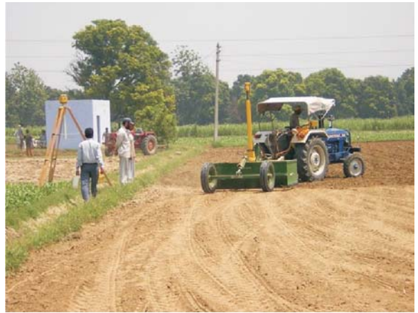
Laser land leveling improves water use efficiency
