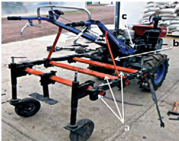
Figure 2. Tool mounting unit. a) Tool mounting bars b) Hitching point c) Power source.
