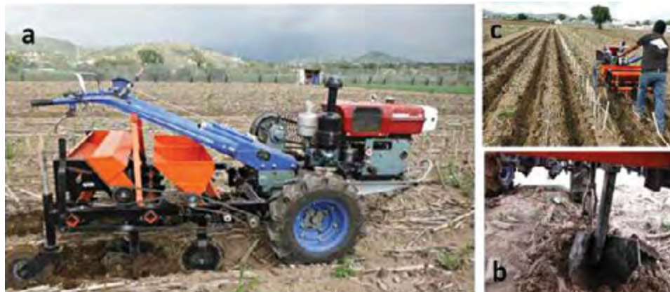
Figure 8. On-field configuration for ridging. a) Full lateral view b) Ridgers in action c) Reshaping the beds.
