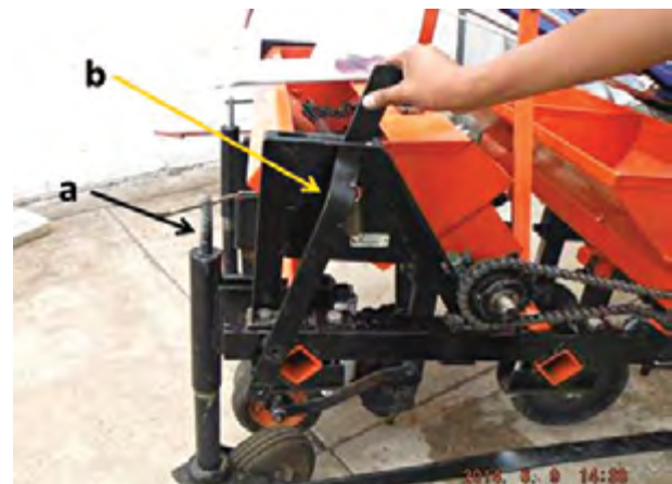
Figure 5. Adjusting transportation/penetration depth wheels and clutch system. a) Transportation wheels b) Clutch handle.
