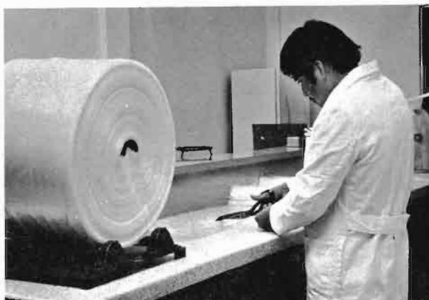
**Figure 9.** The roller device facilitates cutting tubes for borer oviposition cages.
