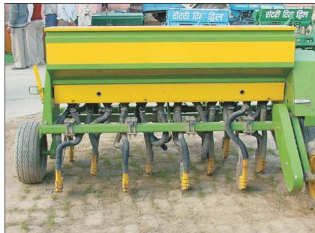
Schematic arrangement of seed-cum-fertilizer tynes on a 3-bar zero till drill
