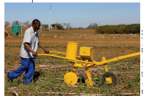
Field calibration and testing of a Grownet direct planter
