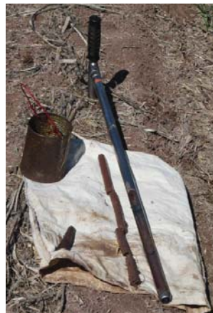
Figure 3. Equipment: soil probe, the soil sample and a can of oil.
