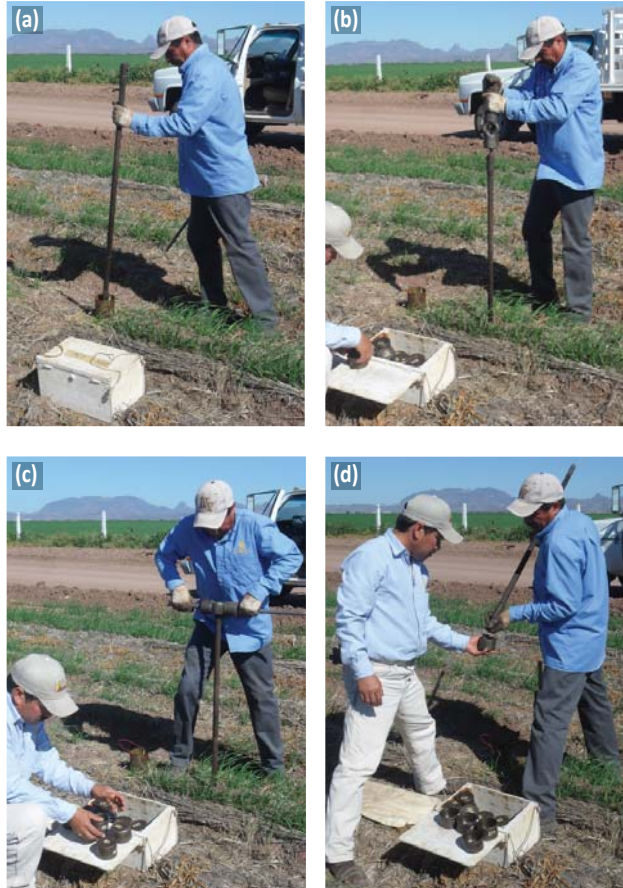
Figure 1. The four steps in sample collection: a) greasing the tip, b) hammering in the probe, c) pulling out the probe, and d) placing the sample in a metal can.
