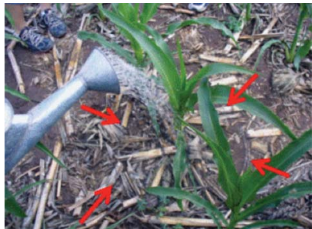
Figure 5. Pouring water at the center of the ring from a height of 75 cm.
