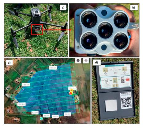
**Figure 2.** (**a**) The DJI Matrice 300 UAV; (**b**) the Mica Sense Altum sensor utilized in this study; (**c**) the flight path plan for the study area image acquisition; and (**d**) the Altum sensor calibrated reflectance panel.
