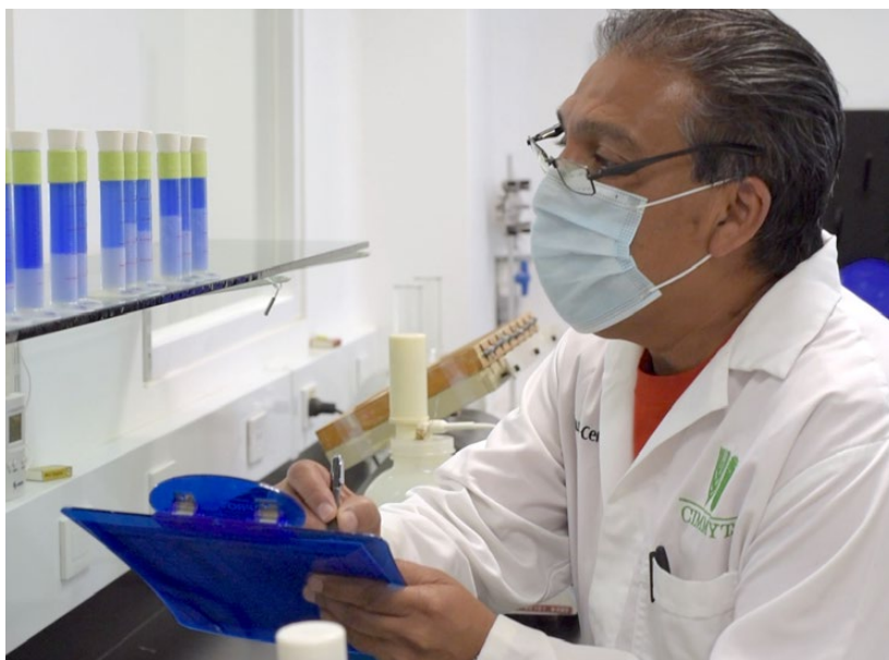
A lab technician determines the sedimentation volume of different wheat flour samples. Larger sedimentation volumes indicate stronger gluten.
