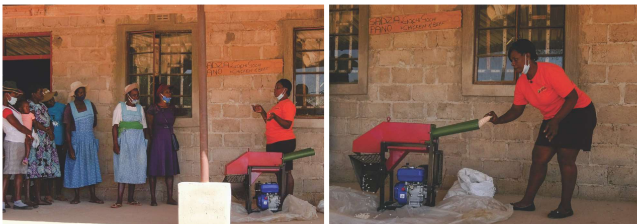
Shelling training and demonstration of shelling procedures with the two-cob maize sheller
