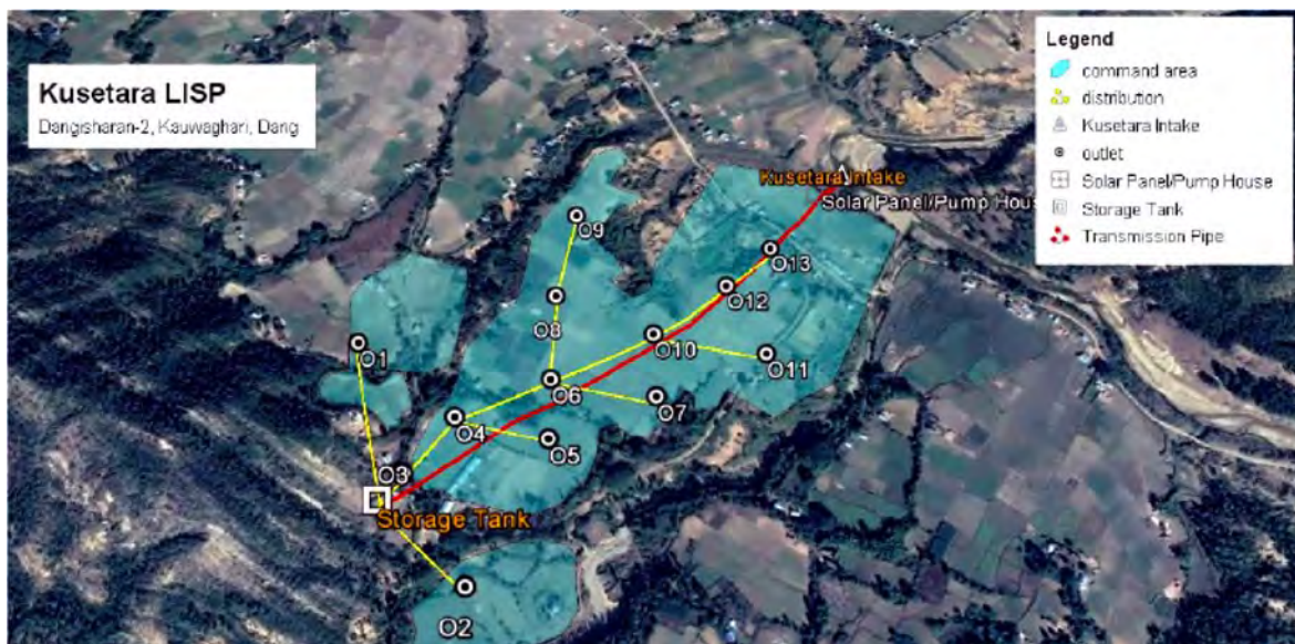
Annex 2-2 (g): Location and associated details of Kusetara Solar Lift Irrigation Project (Source: IMP, 2019) Note: LISP: Lift Irrigation Solar Project
