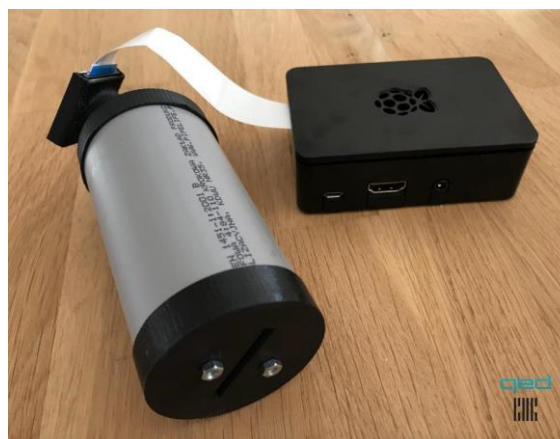
Photo 4.9: Initial prototype of low-cost hand-held near-infrared spectrometer (Credit: William Wu)
