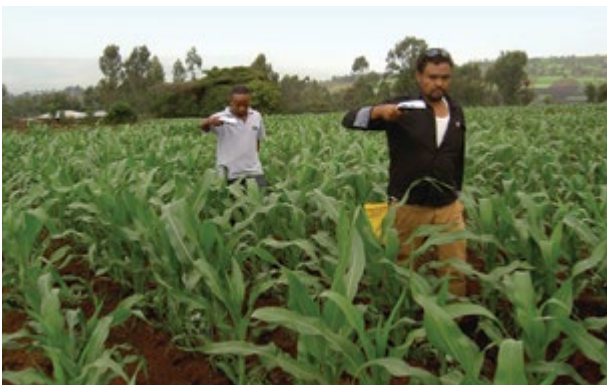
Researchers measuring the NDVI (indicator of leaf greenness) using a hand held GreenSeeker in order to optimize the N fertilizer rate.
