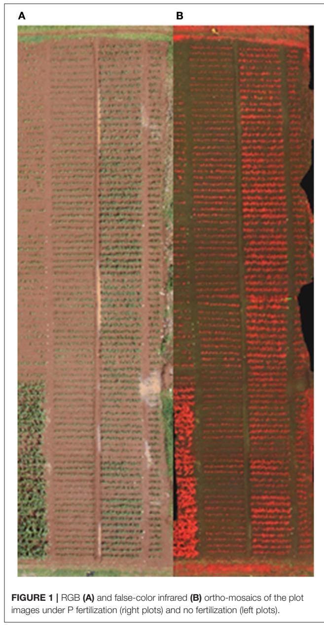
wavelengths in the visible and near infrared regions of the spectrum (MCA12, Tetracam Inc., Chatsworth, CA, US) was also mounted in the drone. The camera consisted of 12 independent image sensors, and optics with user configurable filters. It captured 15.6-megapixels of image data and transferred this to 12 separate flash memory cards. Both RGB and multispectral images were taken at the rate of one every 5 s.
