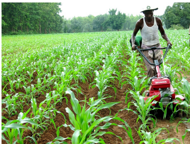
Fig. 5: Simultaneous weeding, inter-culture and earthing-up using ‘power-weeder’.
