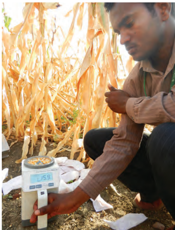
Fig. 12. Measuring grain moisture content.
