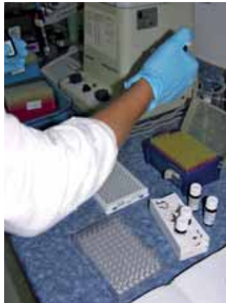
Mycotoxin evaluation using the RIDASCREEN® FAST DON ELISA kit to evaluate the DON levels
