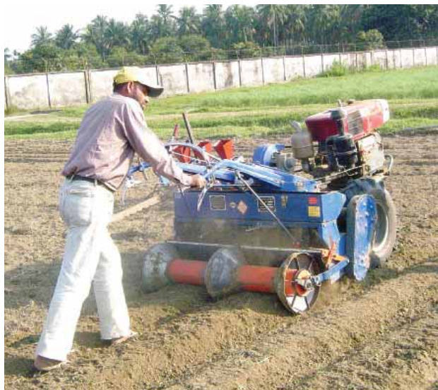
Picture: Soil bed former and planter for light soil being used in Bangladesh. (Source: Enamul Haque, 2003)
