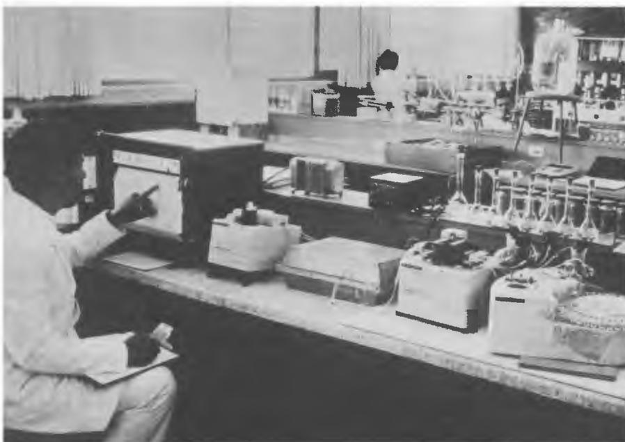
**Modular components of the autoanalyzer working in series.**
