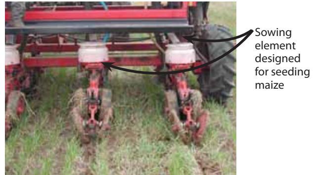
Figure 7. Sowing element of Semeato for maize.
