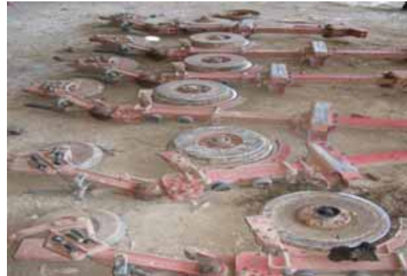
Figure 6. Sowing element of Semeato for wheat.
